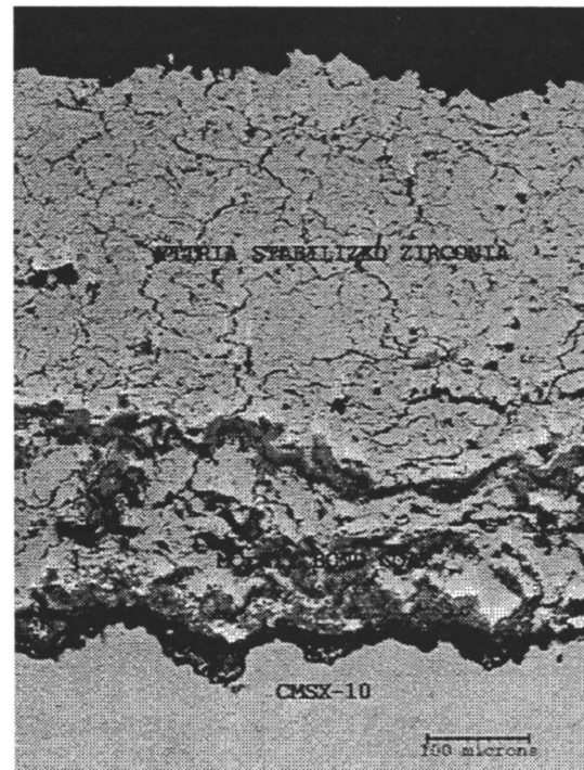
Fig. 7 Air plasma sprayed TBC microstructure on CMSX-10 substrate after thermal cycle testing
