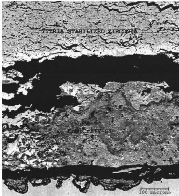
Fig. 6 Air plasma sprayed TBC microstructure on CMSX-4 substrate after thermal cycle testing
